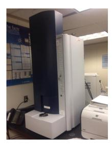
Figure 3: Benchtop Microflex MALDI-TOF mass spectrometer from Bruker Daltonics
